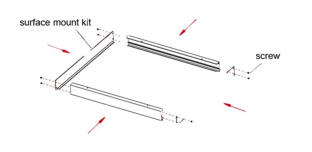
3. Fix the surface mounted frame on the ceiling by using screws.
