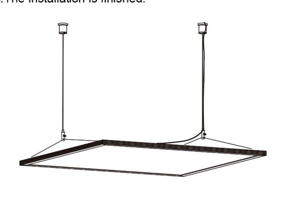
Note: Suspending installation method is not suitable to be used for products with dimensions of 1195\*595mm. 295\*295/595\*295/595\*595/620\*620mm: 2pcs suspension kits needed for installation. 1195\*295mm: 3pcs suspension kits needed for installation.
