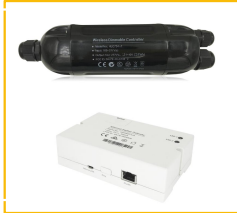
Zigbee wireless controller 1pcs for each luminaire Zigbee gateway 1pcs can control 200pcs luminaire
