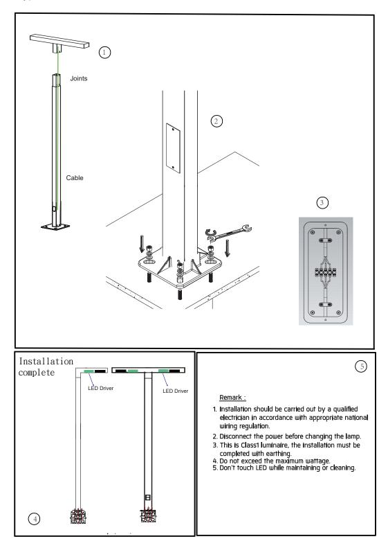
Remark: The fixture must be properly grounded to avoid accidental power leakage and electric shock.
