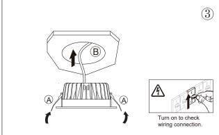
Install the luminaires to the corresponding location and turn on electricity to check wiring connection, light up.
