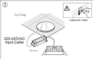
Connect the the load wire into the driver box's driver, and put the driver box into the ceiling as sketch.
