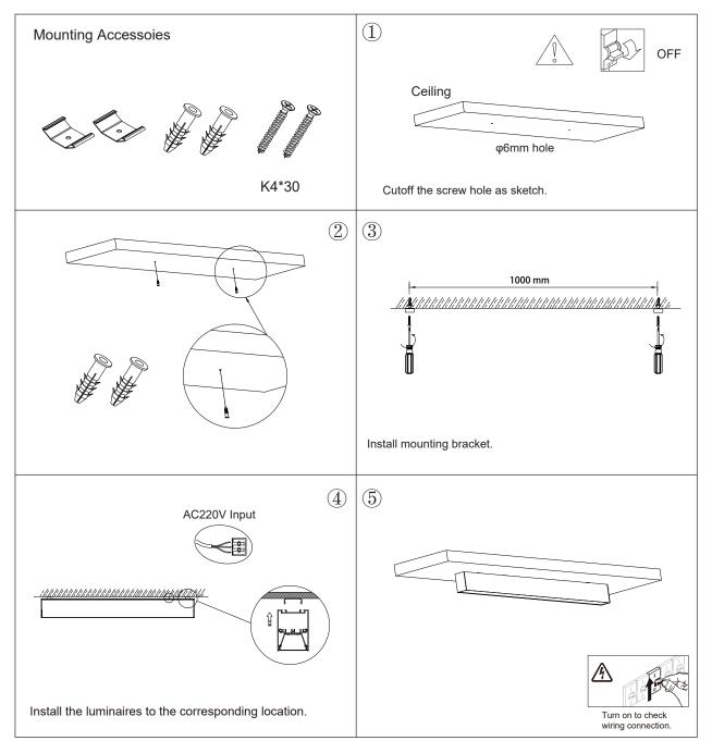
Remark: The fixture must be properly grounded to avoid accidental power leakage and electric shock.
